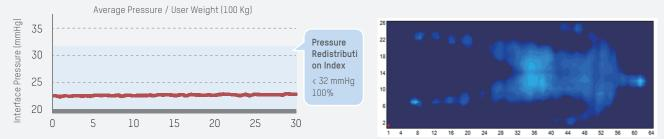
The Pressure Redistribution Index (PRI) and the pressure mapping conducted by placing a test subject weighted 100kg on Verso replacement mattress. The PRI performance is superior as it is far below 32 mmHg at 100% of test period.
