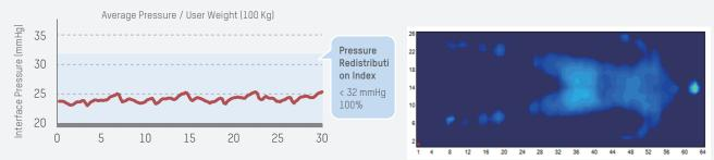
The Pressure Redistribution Index (PRI) and the pressure mapping conducted by placing a test subject weighted 100kg on Verso overlay mattress. The PRI performance is superior as it is far below 32 mmHg at 100% of test period.
